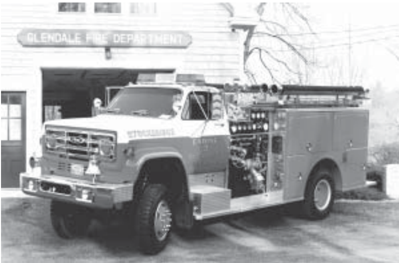
Current Stockbridge Engine 3, Glendale Station, 1986 GMC- Pierce 4 wheel drive 1,000 G.P.M. Pumper
